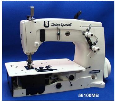
These new white 56100s are distinguished from their predecessors by a new bearing for the left mainshaft. This replaces the bushing used in earlier styles. The bearing handles the load stress at that crucial point much more effectively than a bushing. The bearing allows the shaft to run smoother and cooler. No more downtime or repair labor due to a burned up bushing!
