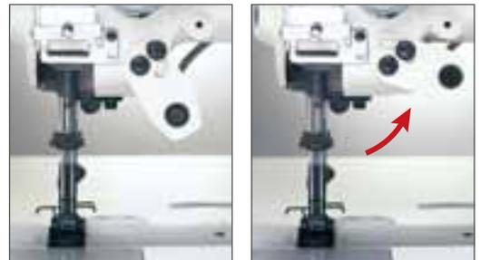
**Bottom-feed micro-adjustment mechanism is provided as standard. (LU-1510N-7, LU-1511N-7)**
