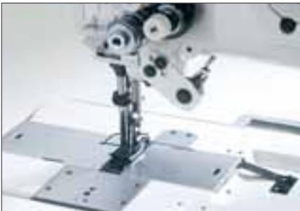
**The walking foot and presser foot's alternating vertical movement can be set and changed with ease.**
